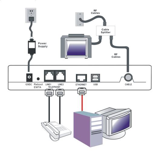
Fig.3: Ethernet Connection
